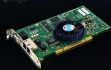
The ZMP-SynqNet Series PC-based controllers provide machine builders with the ultimate in highperformance motion control. The 64-bit ZMP controllers utilize a 466MHz PowerPC processor for optimum flexibility and speed. With a significant increase in processing power, the ZMP family of controllers are available in PCI and CPCI-3U form factors.
